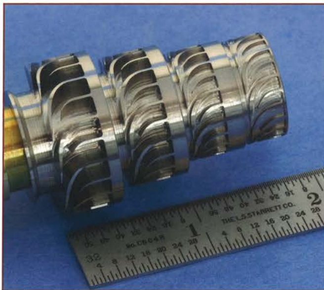
Long-term seafloor testing at 1500 m depth for hydrothermal vent power system (left) and multi-stage turbine impeller for same system (right).
