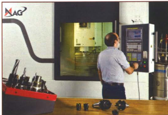
MAG's VMC 960 Machine Tool with a Fully Integrated ICS for Cryogenic Machining.
